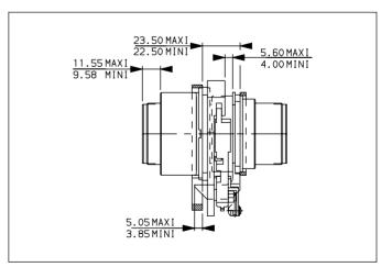
The Launching Security Device is designed to catch the floating connector plug shell during the flight.
