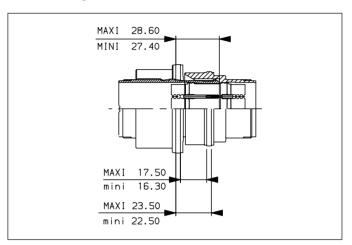
During the mating operation, the receptacle comes up to plug. The front of plug enters in receptacle cone. When plug touches the cone, this induces a lateral movement of plug shell relatively to the flange fixed on panel. This movement stops when the plug shell axis is in conformance with the receptacle ones.
