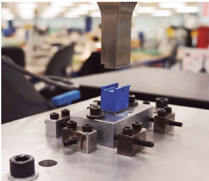
Plastic sonic welding is ideal for combining two molded parts to achieve a robust connector solution
