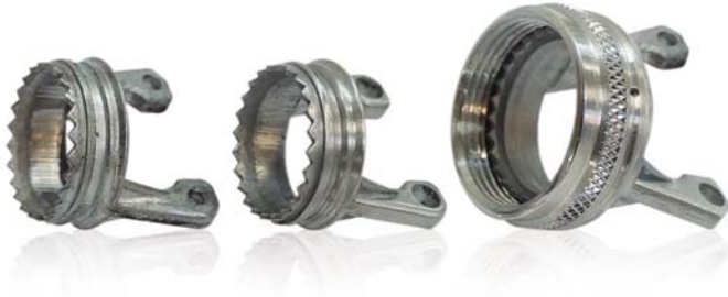
From left to right: die cast part, die cast part after machining, complete assembly
