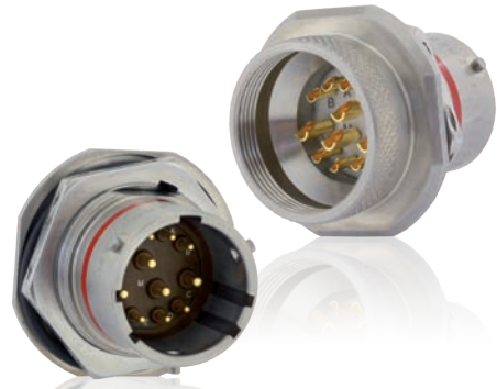
8STA Hermetic Glass bead insulator 1.10^{-7} cm 3 /s hermiticity Low profile design for heat shrink boot
